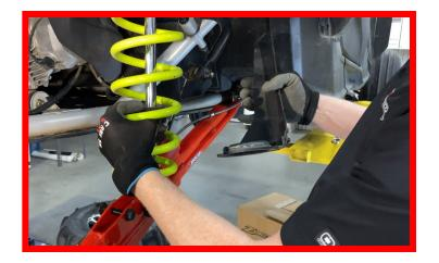
Now slide the spring stack down to completely remove it from the shock body.
