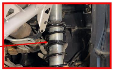
Cross-over Nut will be underneath the Tender Spring.
