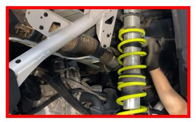
Remove the bottom retainer with guard by lifting up on the Spring Stack providing enough clearance to remove the retainer.
