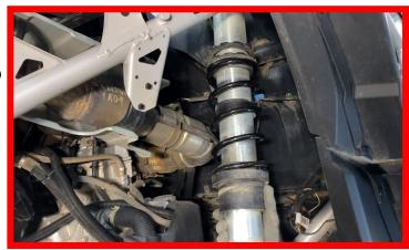
Now slide the NEW ZBROZ Main Spring onto the shock body all the way up to the Spring Divider.
