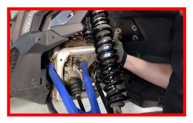
Next Place the lower Spring Retainer back on the same way it came off and then mount your shock back to the A-Arm with the lower shock bolt. Tightening the nut and bolt to factory torque specs.
