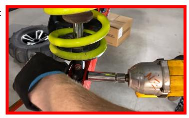
Now back the preload off by grabbing the Spring Stack and rotating it counter clockwise to fully loose.
