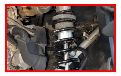
Next Place the lower Spring Retainer back on the same way it came off and then mount your shock back to the Trailing Arm with the lower shock bolt. Tightening the nut and bolt to factory torque specs.
