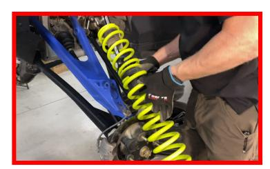
Take the new ZBROZ Tender Spring and place it back on top of the Spring Divider the same direction it came off and slide them back up to the top of the shock body.
