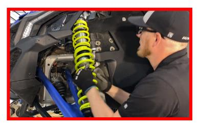
Remove the bottom retainer by pushing down on the wheel hub. You may the an additional person to help you.
