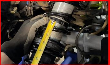
\*Additional Preload may be needed depending on after-market accessories (bumper, cage, tire carrier, stereo system). You can put more pre-load on by repeating turning the pre-load nut more.
