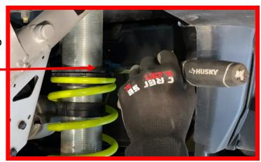
Loosen lower shock bolt on the A-arm. Do not disconnect it from the Trailing Arm at this time.
